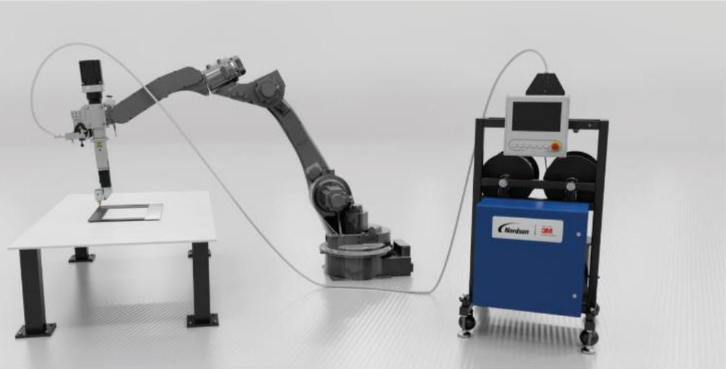
Two sets of Pinch Wheels pull the material off the spool to the applicator/extruder.
